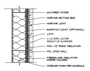
CULTURED STONE OVER SHEATHING WITH METAL STUDS CULTURED STONE OVER RIGID INSULATION WITH METAL STUDS
