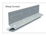
protects these susceptible framing materials. The weep screed also acts to kick the water out from the building and provide the appropriate clearance from grade or a paved surface. In most cases, the weep screed is installed to provide a 4" clearance from grade or a 2" clearance from any paved surface. The weep screed is the first to be installed so that WRB materials can lap over its 3" attachment flange in shingle fashion.
